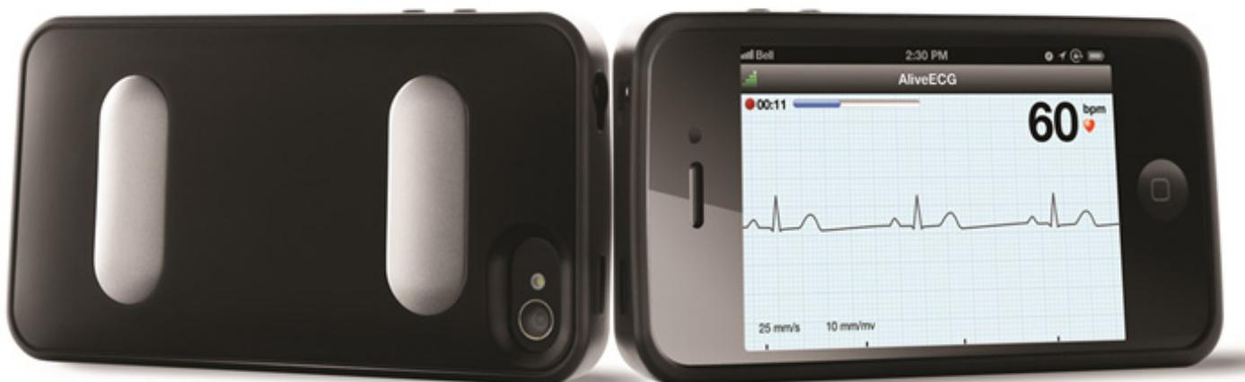
**Figure 1:** The FDA approved AliveCor™ Heart Monitor and application.
