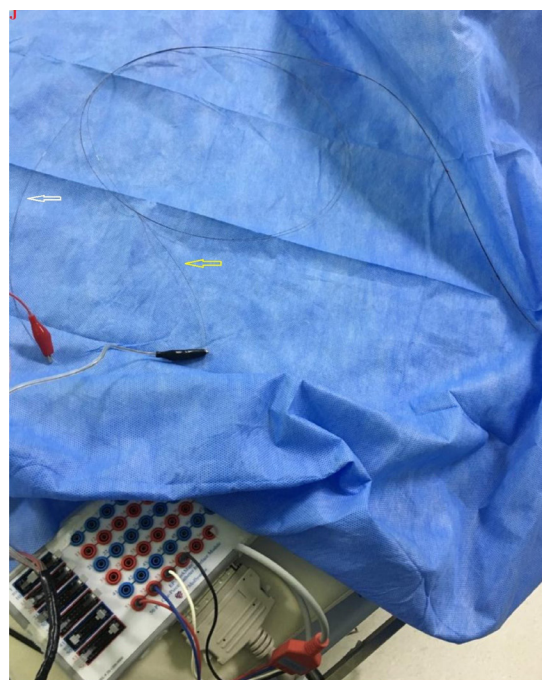
Figure 1J: The inputs of the connection box are connected to the distal tip of whole coronary guidewires (yellow and white arrow) using the recording device
